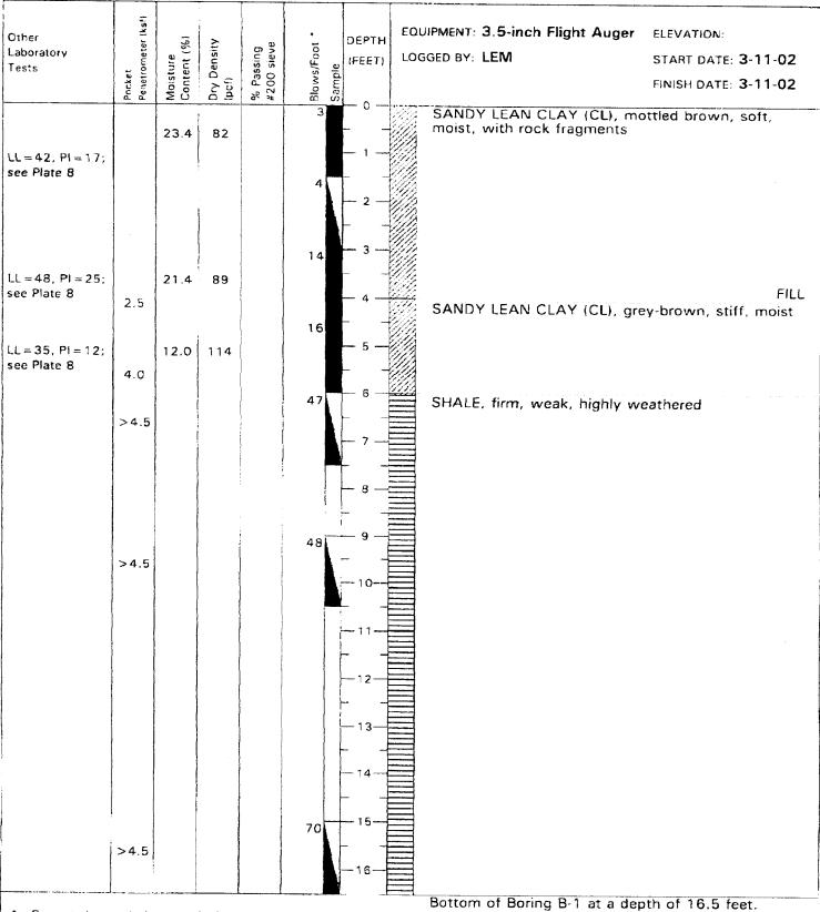
Converted to equivalent standard penetration blow counts.
